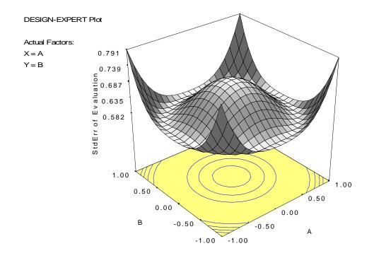
Notice that the plot of the prediction standard deviation has a large "bump" in the center. This indicates that the design will lead to a model that does not predict accurately near the center of the region of exploration, a region likely to be of interest to the experimenter. This is the result of using an insufficient number of center runs. Suppose that the number of center runs is increased to  $n_c = 4$ . The prediction standard deviation plot now looks like this:
