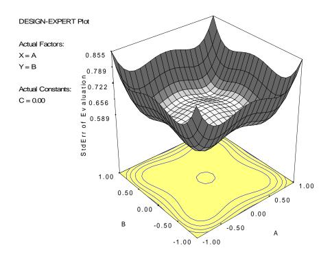
Notice that despite the absence of center points, the prediction standard deviation is relatively constant in the center of the region of exploration. Note also that the contours of constant prediction standard deviation are not concentric circles, because this is not a rotatable design.
