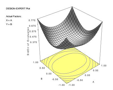
Notice that the contours of prediction standard deviation are not circular, even though a rotatable design was used.
