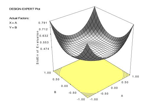
Notice that the addition of two more center runs has resulted in a much flatter (and hence more stable) standard deviation of predicted response over the region of interest. The CCD is a spherical design. Generally, every design on a sphere must have at least one center point or the X'X matrix will be singular. However, the number of center points can often influence other properties of the design, such as prediction variance.
